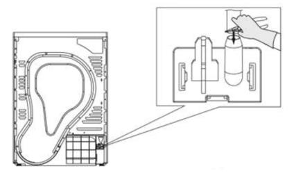
2. Insert the optional bypass hose (using pliers if required), ensuring it is securely in place
