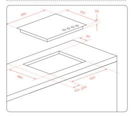
For the purpose of installation and usage, leave a min. of 50mm space surrounding the cut-out. Ensure that the thickness of the work surface is at least 30mm min.
